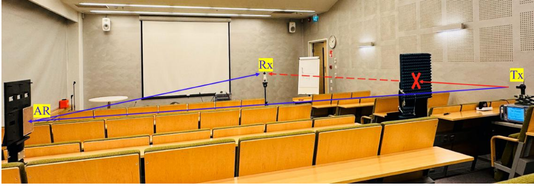
Figure 3: The indoor measurement scenario with an auditorium setting, using a 48 \times 48 -sized AR.
