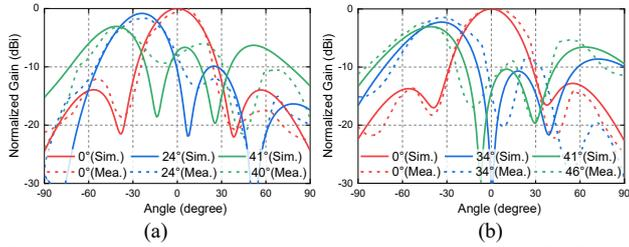
Fig. 11. Simulated and measured beam steering patterns at 14.5 GHz. (a) Vertical polarization. (b) Horizontal polarization.
