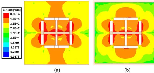
Fig. 7. E-field distribution at the middle layer at 28 GHz. (a) without metallic via wall. (b) with metallic via wall.
