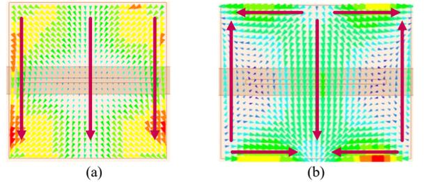
Fig. 6. J current distribution of each radiator shape at TM 21 mode. (a) Square. (b) Rectangular.
