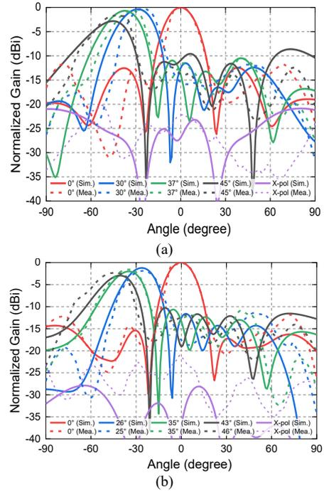
Fig. 13. Simulated and measured beam steering patterns at 28 GHz. (a) Vertical polarization. (b) Horizontal polarization.
