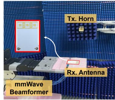
Fig. 12. Measurement environments of Ka-band radiation pattern.
