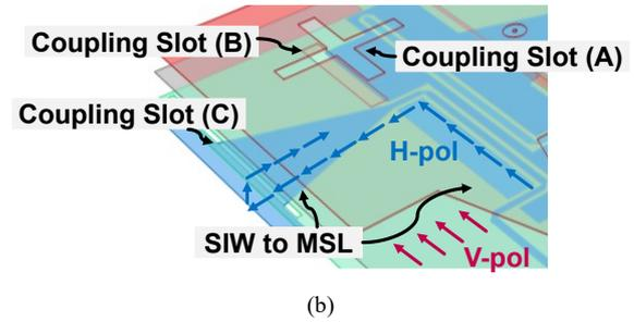
Fig. 9. (a) Exploded view of the Ka-band dual-polarized antenna. (b) Interconnection structure of the Ku/Ka-band dual-polarized antenna.
