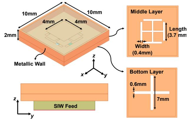
Fig. 4. The proposed Ku/Ka dual-polarized unit element.
