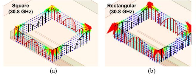
Fig. 5. E-field distribution of each radiator shape at TM 21 mode. (a) Square. (b) Rectangular
