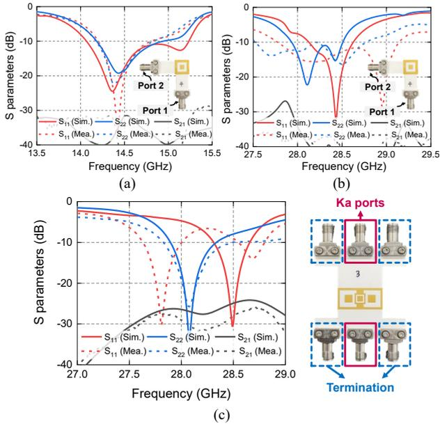
Fig. 10. Simulated and measured S parameters. (a) Ku-band of Ku/Ka antenna. (b) Ka-band of Ku/Ka antenna. (c) Central Ka-band antenna.
