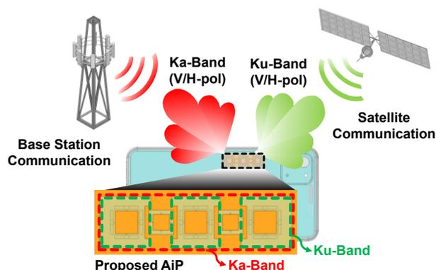
Fig. 1. The conceptual illustration of the proposed Ku- and Ka-band dual-polarized antenna-in-package within mobile devices for terrestrial and satellite communications.
