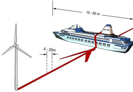
Fig. 4. Turbine optical shadowing and partial shadowing of large vessels °
