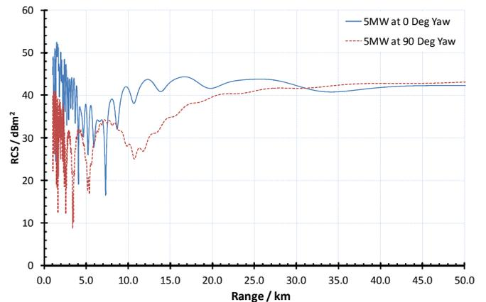
Fig. 2. 5MW Turbine nearfield RCS variation with range at yaw angles 0° and 90°
