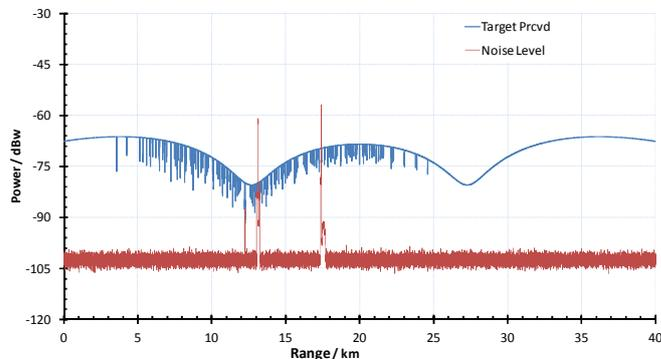
Fig. 8. Power received from the modeled vessel along the modeled route
