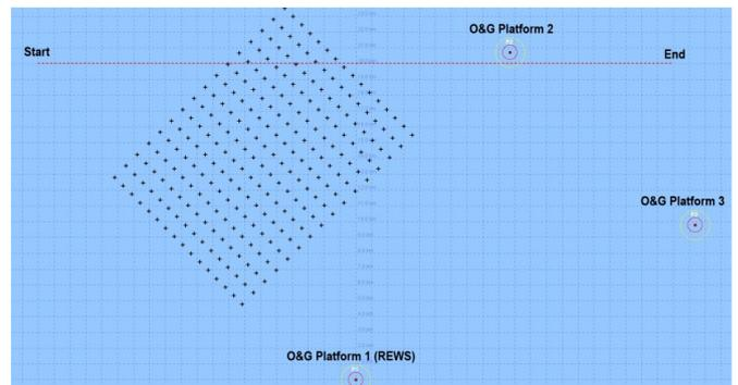
Fig. 1. Modeling layout of the wind farm, REWS, the O&G platforms and the proposed vessel route
