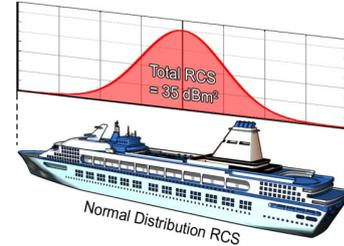
Fig. 6. Vessel RCS as multiple points normally distributed along the vessel length
