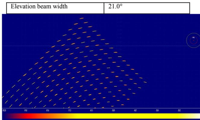
Fig. 7. Power received from the wind farm on a scan converted PPI display
