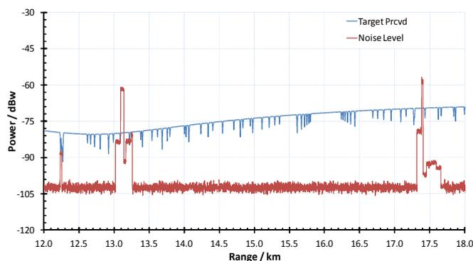
Fig. 9. Details of the effects of shadowing on power received by the vessel vs. the returns of the wind farm
