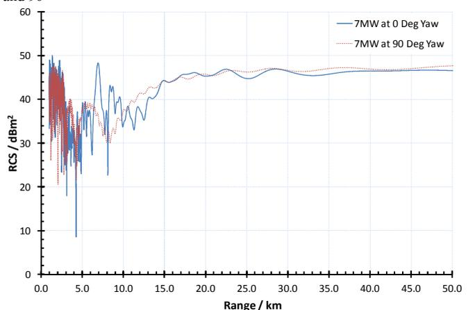
Fig. 3. 7MW Turbine nearfield RCS variation with range at yaw angles 0° and 90°
